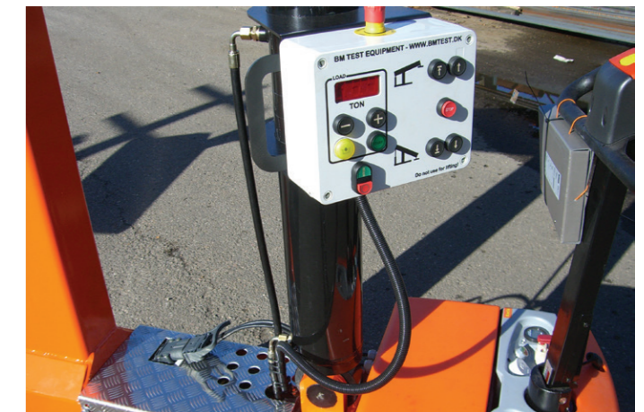
The control panel can be turned to ensure the best possible position while operating it.
