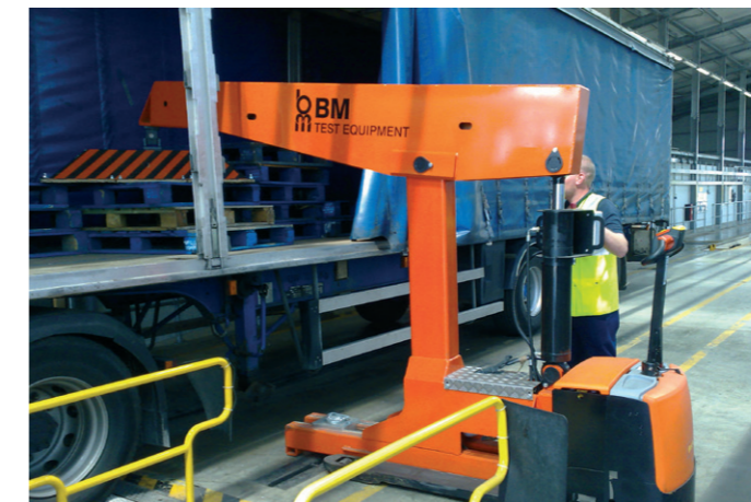
The control panel can be turned to ensure the best possible position while operating it.
