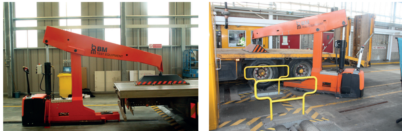
BM74000 placed in position behind or from the side of the vehicle
